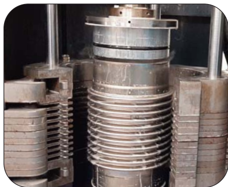
Thorburn's Precision hydro formed bellows manufactured with various ply thicknesses
