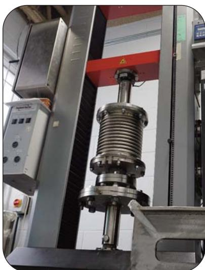
Metal bellows cyclic fatigue testing
