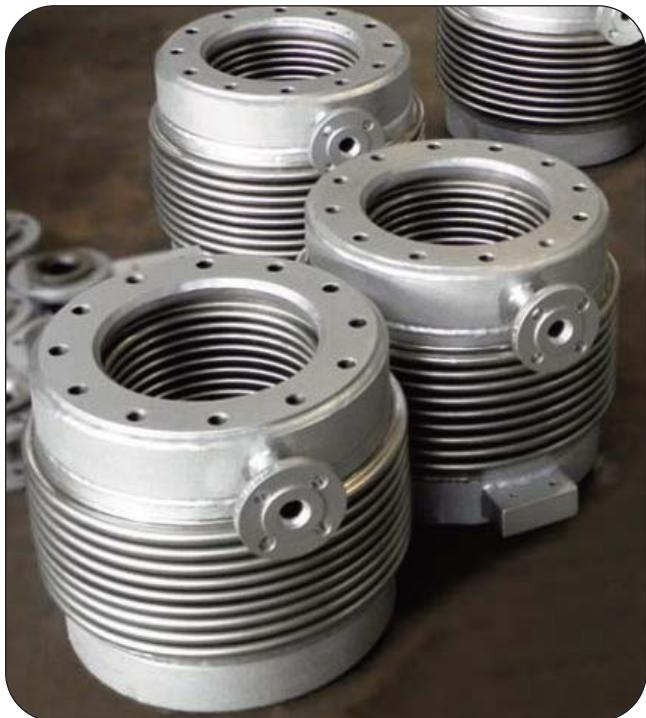
Jacketed bellows consist of a single bellows with another larger bellows mounted around it forming a chamber between the two bellows. Fluid is circulated between two bellows through inlet and outlet connections attached on the outer pipe on opposite sides of the bellows 180° apart. The media going through the inside bellows is kept under a fixed temperature by passing another liquid on the outside bellows. This facilitates heat exchange through thermal expansion of the pipe.
