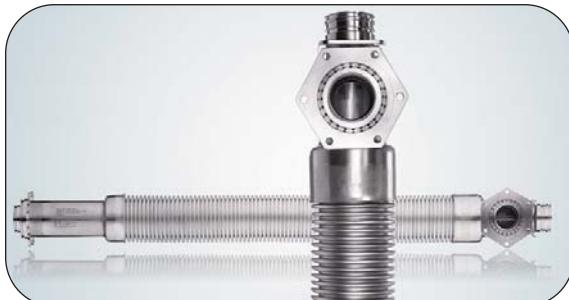
Bellows for trim tank kerosene lines connects the rigid transfer pipe to the flexible trim tank in the horizontal stabilizer and enables continuous drainage and leakage detection for the inner fuel line
