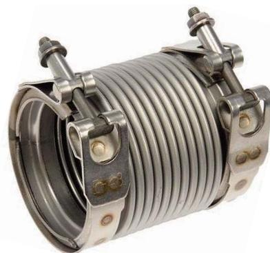
Automotive exhaust pipe metal bellows
