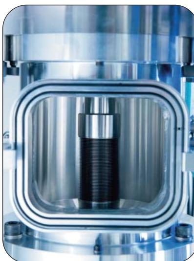
Helium leak testing metal bellows
