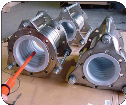
Thorburn's Hot-Flex expansion joint PTFE liner undergoing a 10,000 Volt spark test to detect perforation
