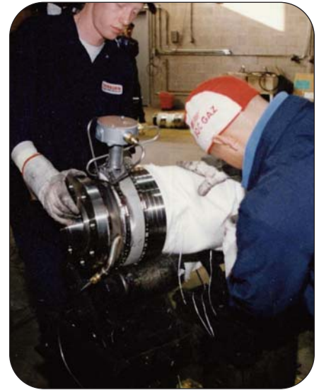
Installing inner insulation on Sure-Temp™ hose
