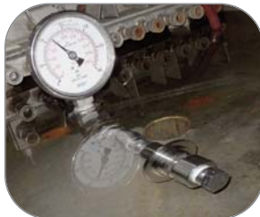
Pneumatic test at 100 psi
