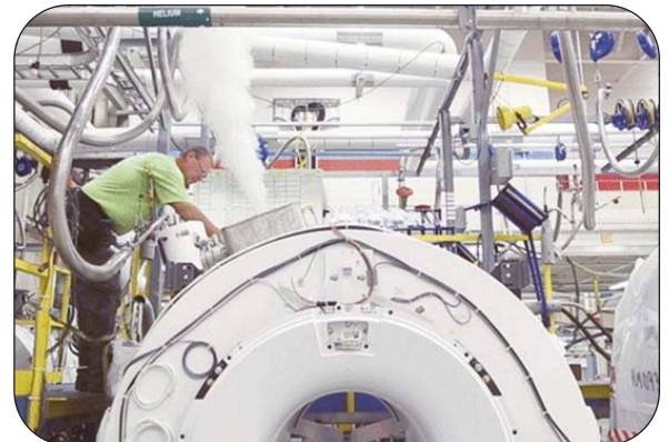
Thorburn's Met-O-Seal Series MTS4 hose coupling used for loading liquid helium in an MRI machine at -269°C (-452°F) just above absolute zero. Magnets at that temperature lose all electrical resistance and become superconducting thus produce the same magnetic field for a thousand years with no more power required.
