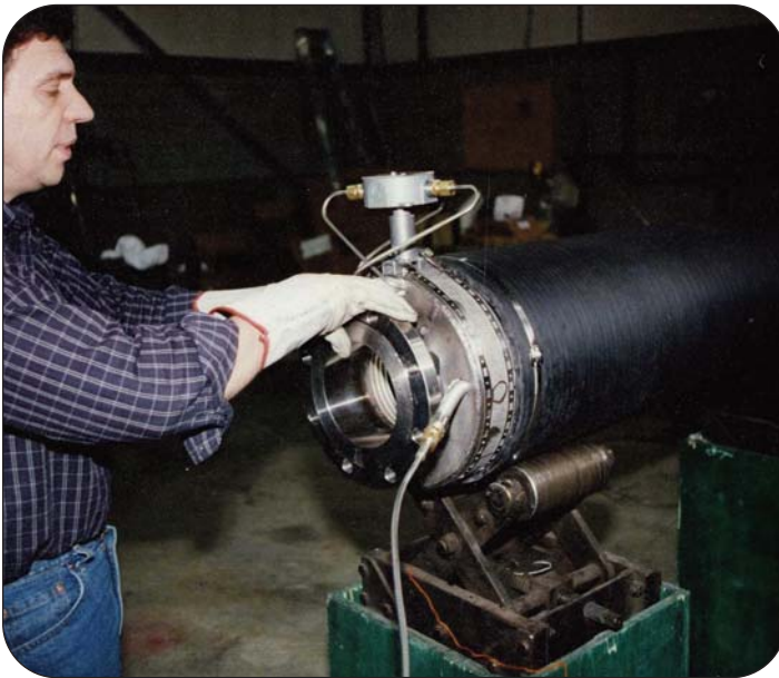
Manufacturing Sure-Temp™ electrically heated hose assembly
