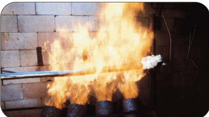
Thorburn's Ball Joint Armor-Flex™ tested at 1100°C
