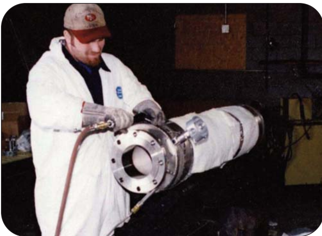
Performing quality check of Sure-Temp™ hose
