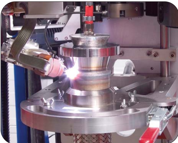
Automated fitting to end joint orbital welding
