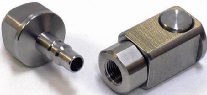
(N)T11 - Quick-release couplings for remote handling of circuits in confinement cells & glove boxes. The long range guiding allows a pre-guiding of the plug into the socket for an easy connection and disconnection.
