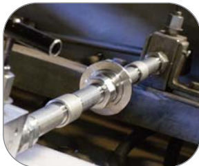
Hydrostatic test at 4000 psi
