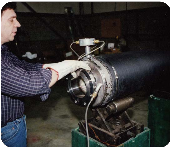
Manufacturing Sure-Temp™ electrically heated hose assembly
