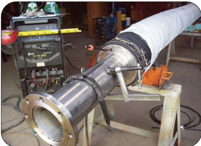
Custom end fitting on Sure-Temp™ hose assembly
