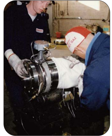
Installing inner insulation on Sure-Temp™ hose
